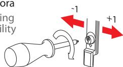
Positioning of the top and bottom hinge body
